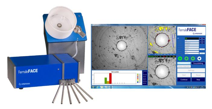
FERRULE FACE supports fully automatic and high efficient Ferrule end-face inspection. With the help of auto feeding, auto inspection and auto classifying functions, FERRULE FACE can easily test more than 3000 pieces of ferrule per hour, minimal human intervention is needed. FERRULE FACE is a must-have instrument for ferrule manufacturer; it's the guarantee for high quality and efficiency.
