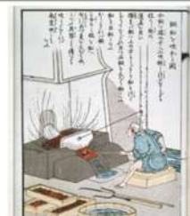
Sumitomo's original copper refining method
